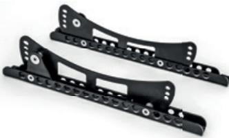
**EB5** This 3 mm steel Elise/Exige specific bracket set is made for fitting either a B6 Screamer, B7, or B6-43 XL Screamer seat to the original Lotus runners. They allow the driver to adjust the angle and height of the seat. They also have mounting points for the original seat belt mountings.
