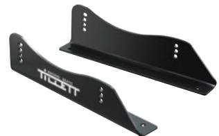
**TB3** side mounted brackets are a 30 mm taller version of the TB2. It is sometimes necessary to lift the seat in a saloon car as the B5 driving position is very low when compared to regular seats. TB3 brackets are 90° and therefore can point inwards or outwards. **1.36 kg**
