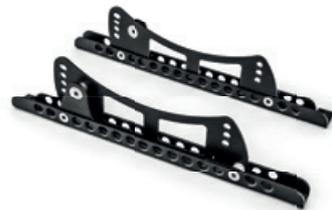
**EB2** This 3 mm thick steel mounting bracket set is designed to fit directly on top of the existing Elise/Exige runners and allows the driver to adjust the angle and height of the B5 seat. They also have mounting points for the original seat belt mountings. **1 kg**
