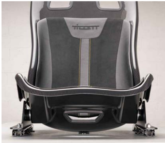
When on the lowest bracket setting using the spacers there is a 2 mm gap to a flat floor
