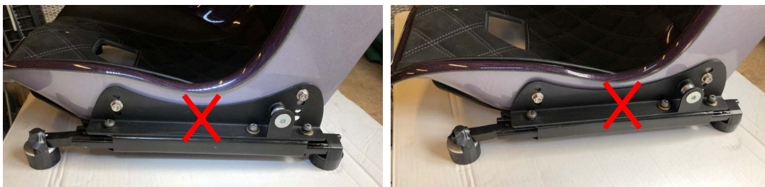
These positions do not allow handle operation
