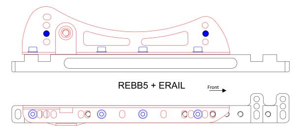
The setting above is for an REBB5 to fit a B5 seat positioned for a tall driver, or for a passenger seat that is required to be set towards the rear.
