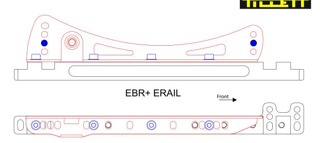
The setting above is for an EBR bracket to fit a B6, B7, B8 and B9 seat positioned for a tall driver, or for a passenger seat that is required to be set towards the rear.
