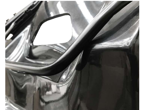
Using the lower front holes for angle adjustment will cause conflict between the seat base and the handle of the Lotus OEM runners.
