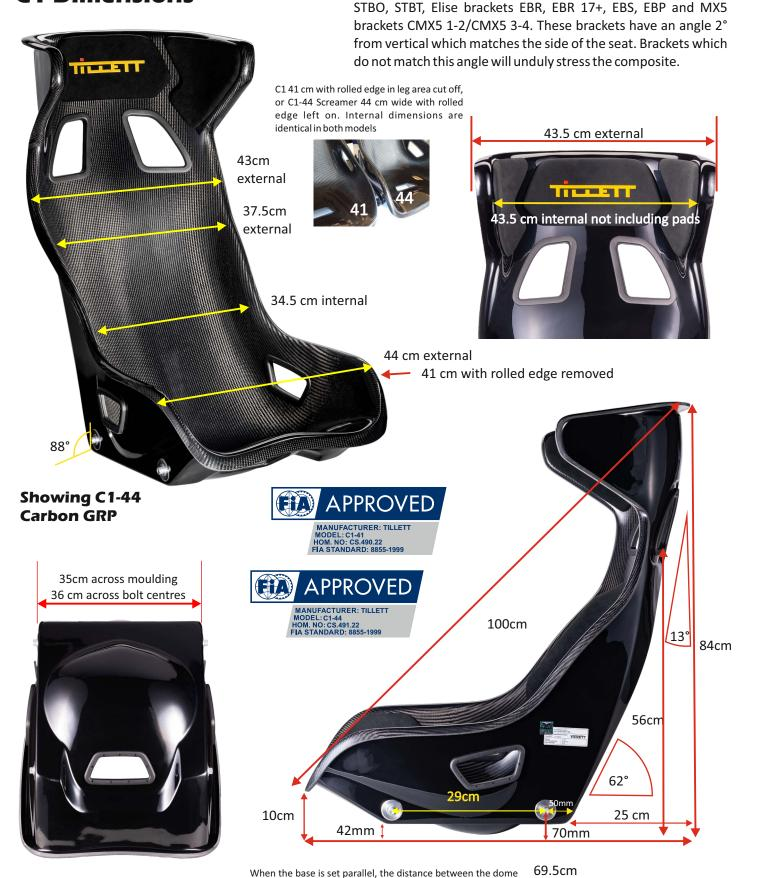
on the bottom of the seat and the mounting frame is 42mm.
