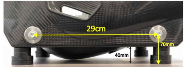
When the base is set parallel, the distance between the dome on the bottom of the B7 XL seat and the mounting frame is 40mm.
